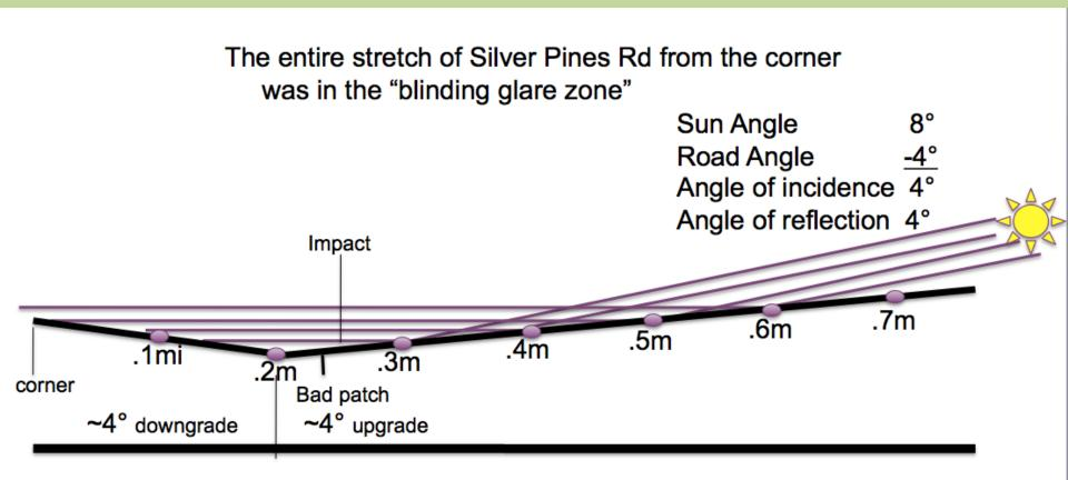
The re-enactment lighting was off by only 3 degrees Azimuth & elevation. What the lighting the day of the accident would have been like from the second CLARK turned onto Silver Pines Rd would have been this...
